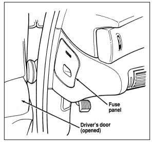
The instrument panel fuse panel location
